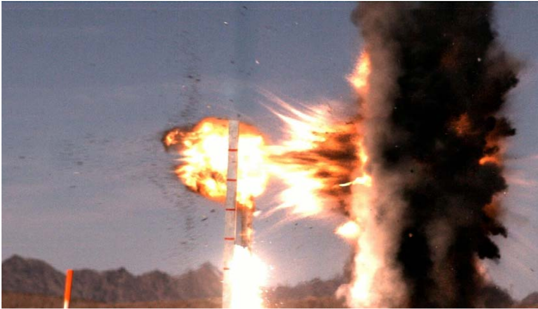
Full-scale test of Northrop-Grumman's Integrated Army Active Protective System (IAAPS), featuring the inert-fragment explosive warhead designed and built by DE Technologies. When the projectile reached the location of the dark cloud, the warhead was detonated, to project the pattern of inert-metal fragments visible on the left.
