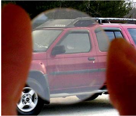
Figure 1. Transparent CeraLumina™ disk (~2mm thickness) with high in-line transmittance.
