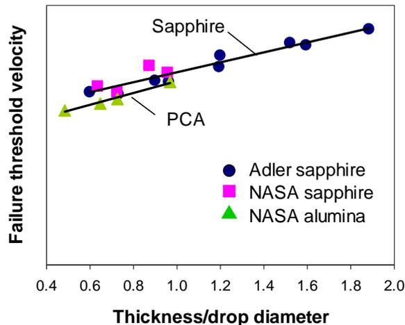
**Figure 3.** Results of single drop water impact tests (normal incidence) show similar performance for polycrystalline alumina and sapphire. All tests were conducted at NASA-Marshall Space Flight Center. “Adler sapphire” is data generated previously by Adler using the same test equipment. “NASA sapphire” is sapphire tested by NASA to compare with Adler’s data. “NASA alumina” is CeraLumina™ tested by NASA.
