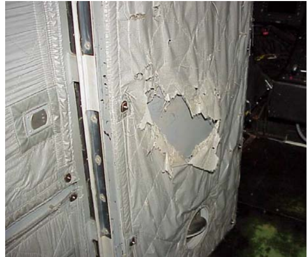
Quilted insulation blankets installed with click-studs bonded to the airframe.
