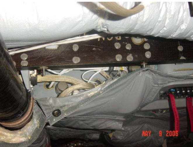
Quilted insulation blankets installed with click-studs bonded to the airframe.
