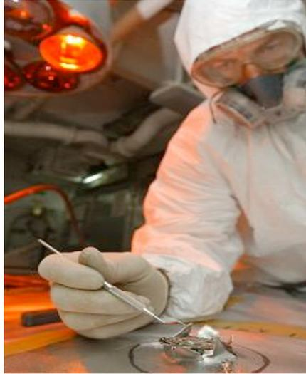
Wing damage repair on-board ship. Carriers have facilities for both sheet metal and composite repair.
