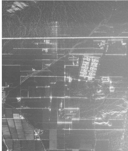
Figure 1.6: SAR image created using a TSC-generated, spectrally-compliant waveform
