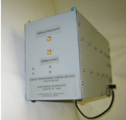
Prototype SHF Shipboard Cosite Interference Canceller; Protects SLQ-32 EW Rx from SHF SATCOM RFI
