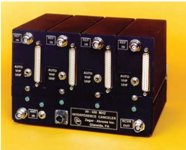
Figure 3: Figure ZA's Frequency Hopping Adaptive Interference Canceller (HAIC™)
