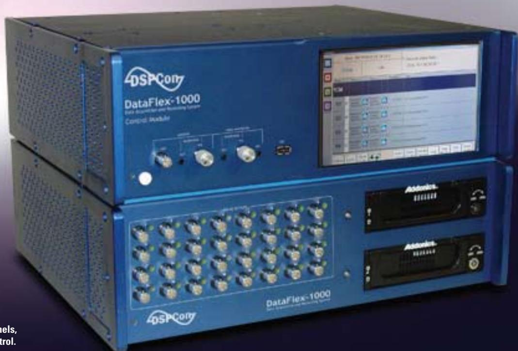
DSPCon's DataFlex solutions offer unlimited channels, built-in signal conditioning, and touch-screen control.
