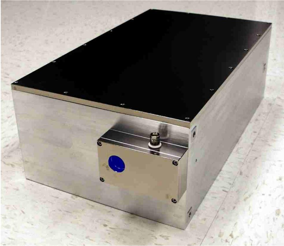
*Figure 1 – Photo of JP Innovations, LLC eye-safe laser head that has been environmentally tested and operates over a wide range of temperature conditions on a mobile platform. The blue laser under development will have a similar size and geometry to this laser.*
