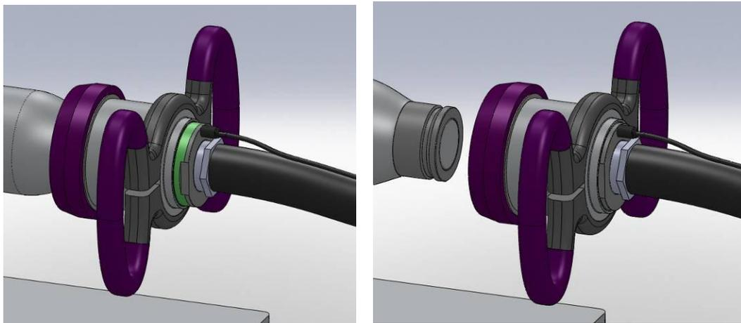
**Figure 2, Fueling nozzle connected, ready for fueling (left) and disconnected (right)**
