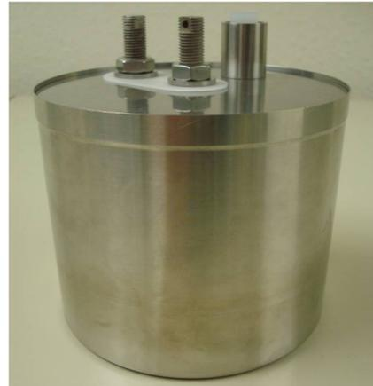
**Figure 1: QynCap prototype, can is 4.5" diameter × 4.75" high**
