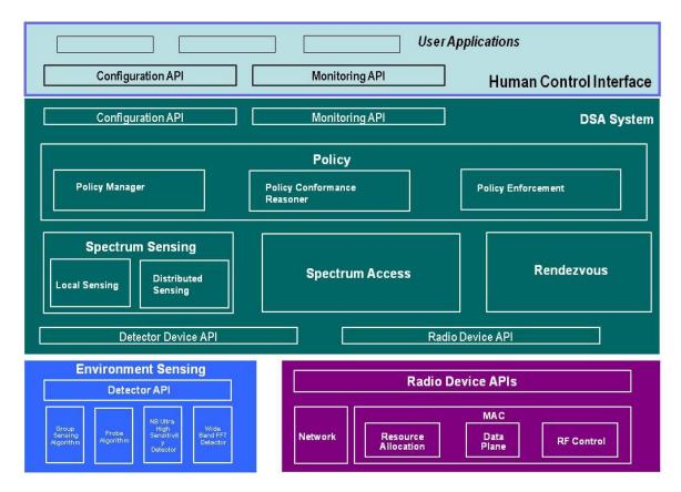
Figure 1. Existing SSC DSA Software Architecture for Software Defined Radios
